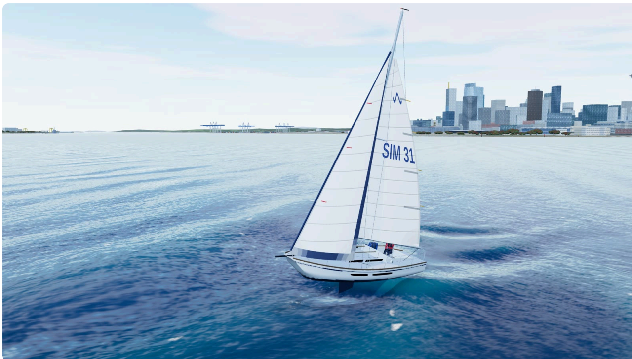
Figure 9.3 The same boat in a stronger wind, with a reef in the mainsail and some of the jib rolled away: upright, and faster.
