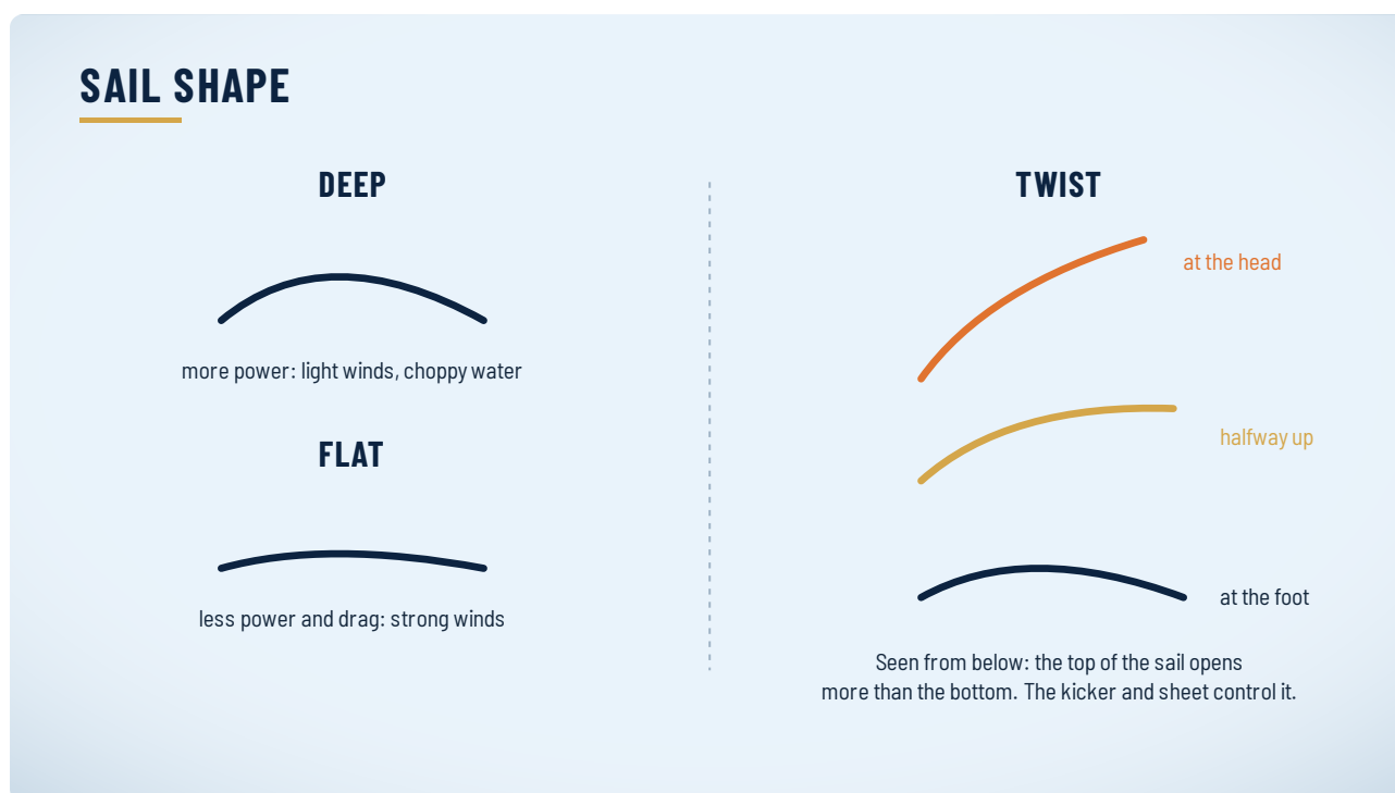
Figure 4.6 Depth and twist. A deep sail gives more power; a flat one less. Twist opens the top of the sail to spill wind.
